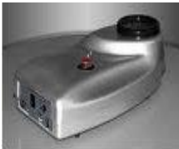
Figure 1: Photograph of GDV Camera pro version 3 designed for measuring one finger at a time.
